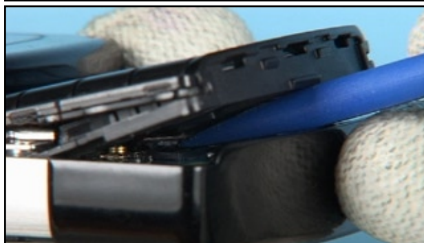
16. Disconnect this flex foil connector.
